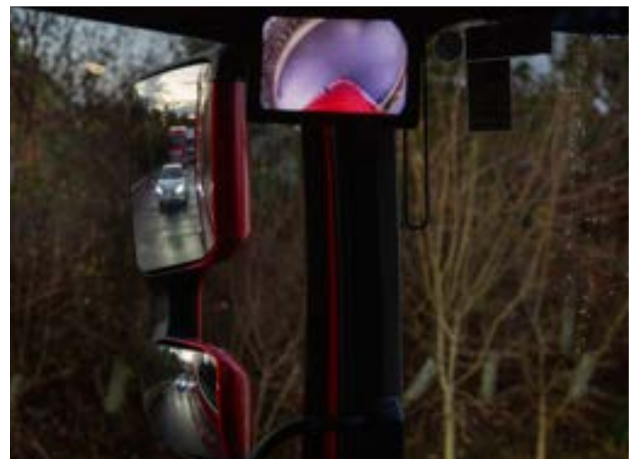
The camera monitors contain an inbuilt light sensor (top) helps maintain image brightness even in low light conditions.
